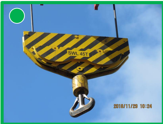
Block in good condition and safety latches operational
