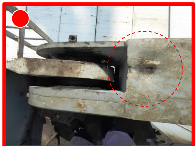
Heavy indentation on jib top plate near pivot point
