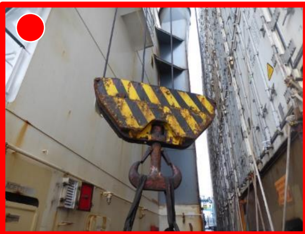
Block with excessive corrosion
