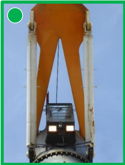
Luffing cylinders with spot corrosion
