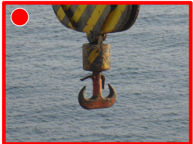
Safety latches inoperable
