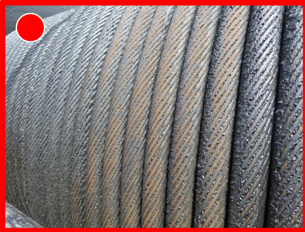
Wire with corrosion
