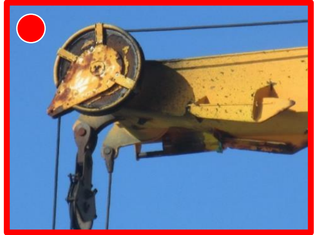
Jib end sheave with excessive corrosion
